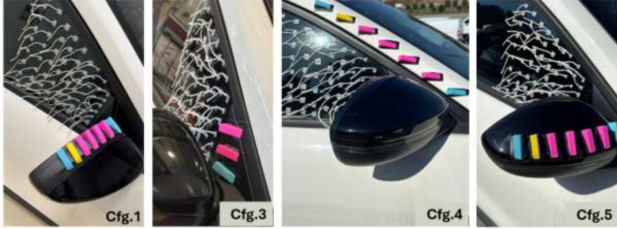
Figure 1. Physical placement of the add-on vortex generators for Cfg.1, Cfg.3, Cfg.4, and Cfg.5.
