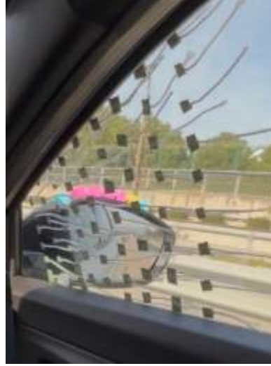
Figure 4. Tuft motion pattern at an instant during the measurement of Config1.
