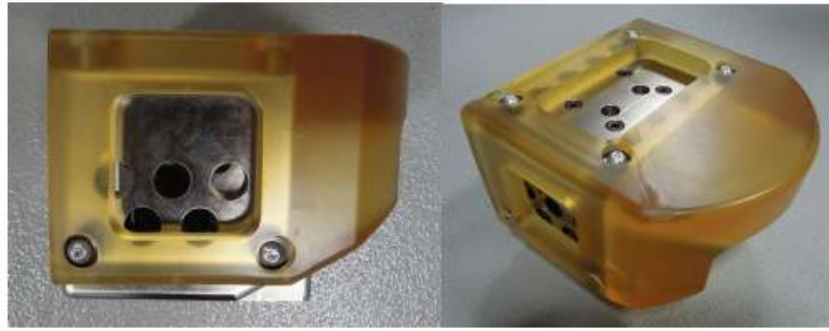
Figure 3.7 Bolt-on upper body part (7 kg) in FlexPLI-UBM
