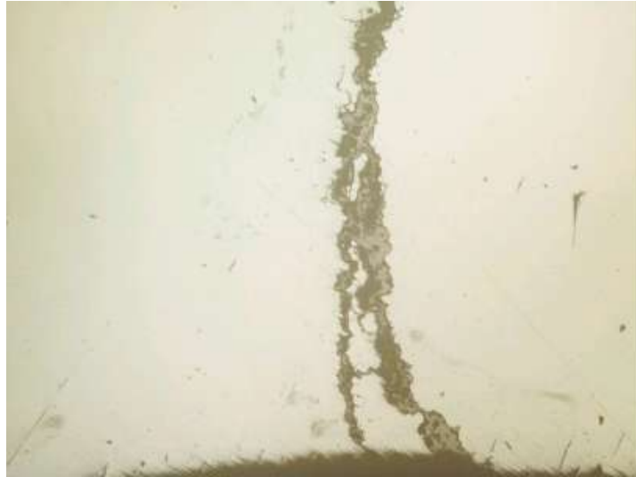
Figure 8. MPI crack control results in direct quenching in brine media
