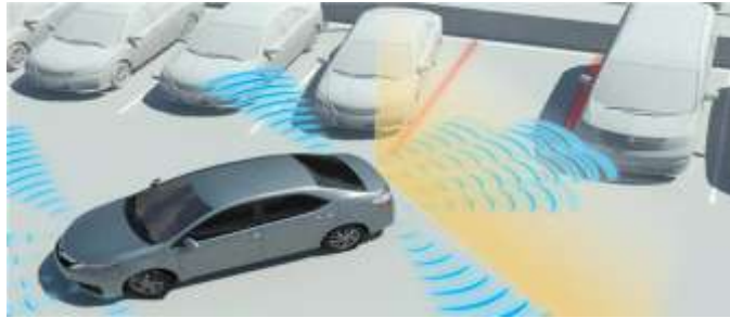
Figure 1. Parking sensor coverage areas during parking [5]
