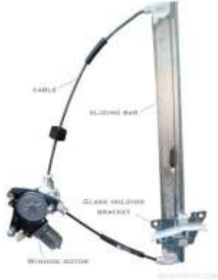
Figure 4. Single rail window system
