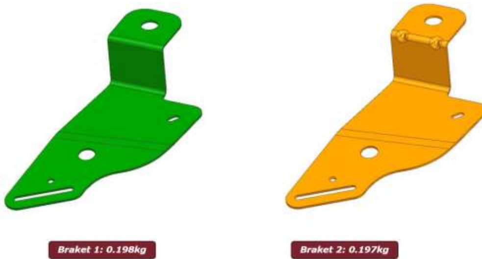
Figure 3: Bracket 1 and Bracket 2 model and weight
