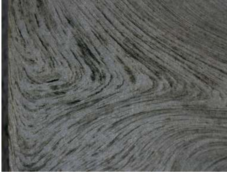
Figure 13. Fiber flow for direct quenching in oil media
