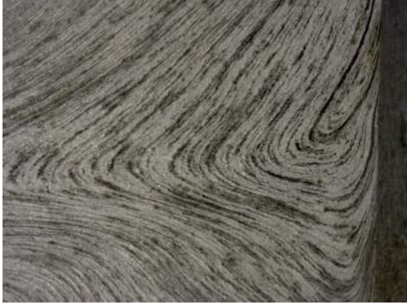
Figure 11. Fiber flow for direct quenching in polymer media
