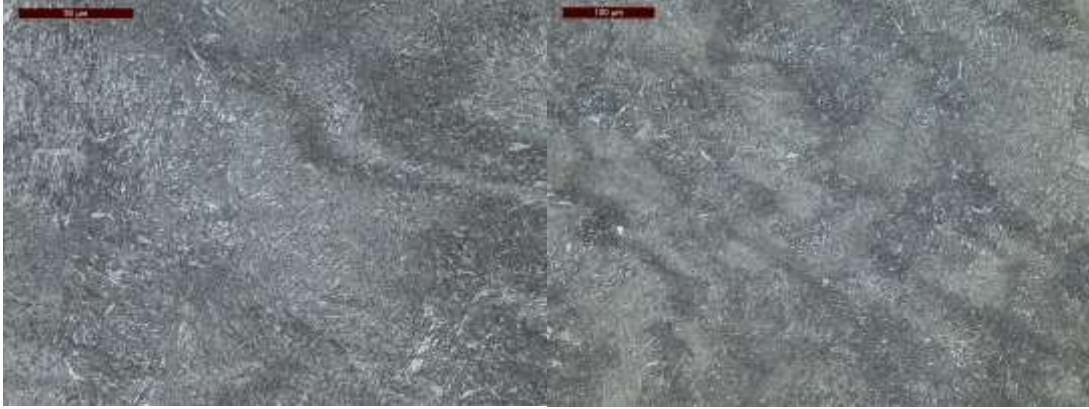
Figure 1,2: Direct quenching of polymer media microstructure results
