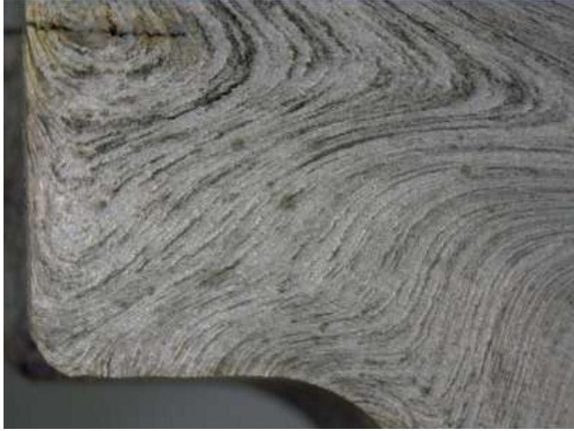
Figure 12. Fiber flow for direct quenching in brine media
