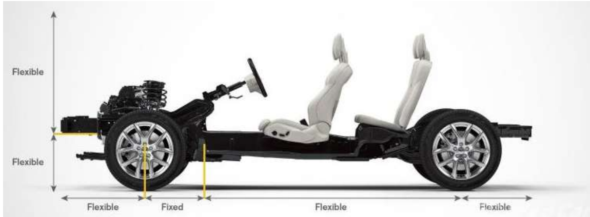
Figure 1. A typical modular vehicle platform illustrating fixed and flexible zones. Notably, the distance between the steering rack, foot pedals, and engine compartment remains fixed, ensuring consistent driver ergonomics across different vehicle models[12]
