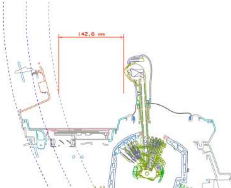
Figure 10 Section view of the relocated gear selector with reach curves
