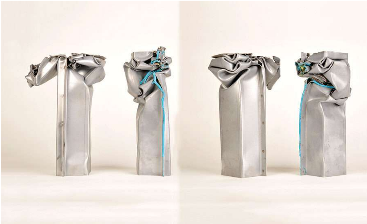
Şekil 1. (Figure 1. Left: structure built without adhesive; Right: 0.2 mm thinner structure built with adhesive)
