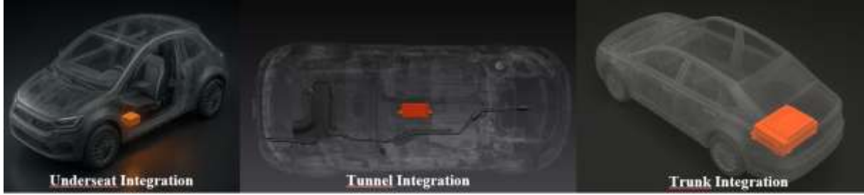
Picture 4. MHEV Battery Placements
