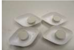
Figure 1: Desired compacted bentonite samples.
