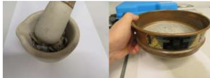
Figure 3: Mortar with purified bentonite and 300 µm sieve.
