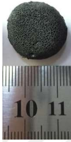
Fig.2. Preform produced using SiC and volatile components
