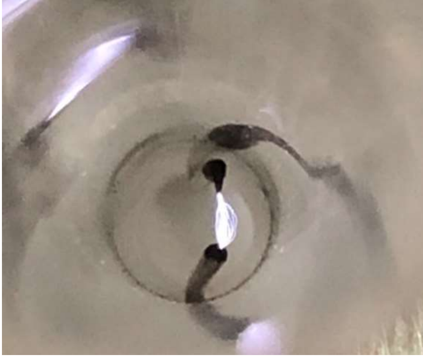
Figure 3.1 : Image of the discharge inside the quartz glass tube.
