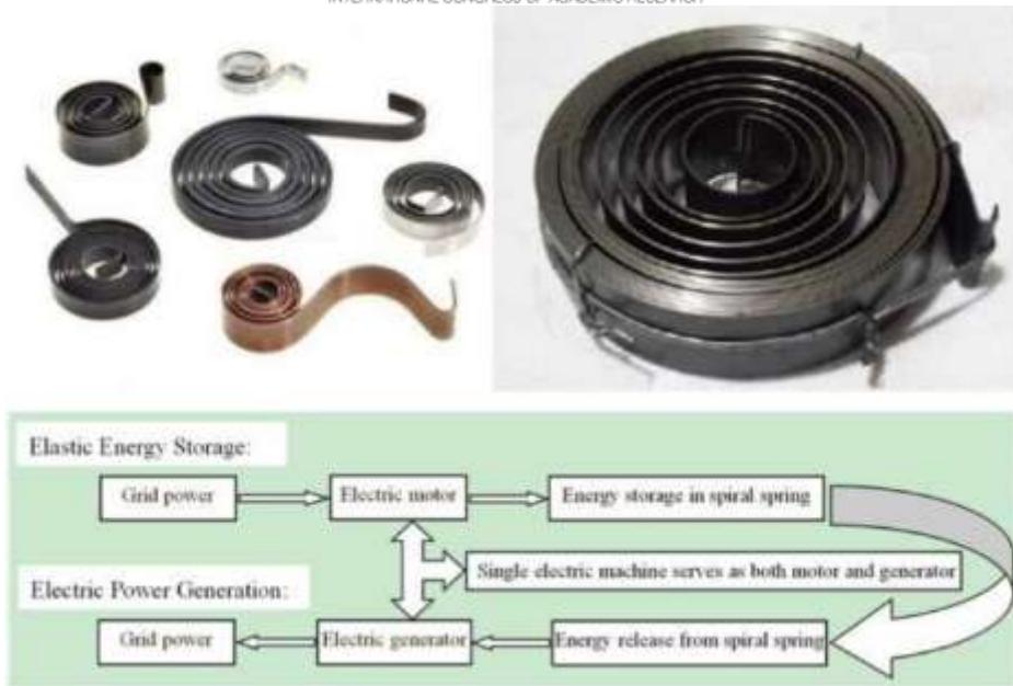
Figure 2. Spiral spring types and energy flow (Guo et al., 2023)
