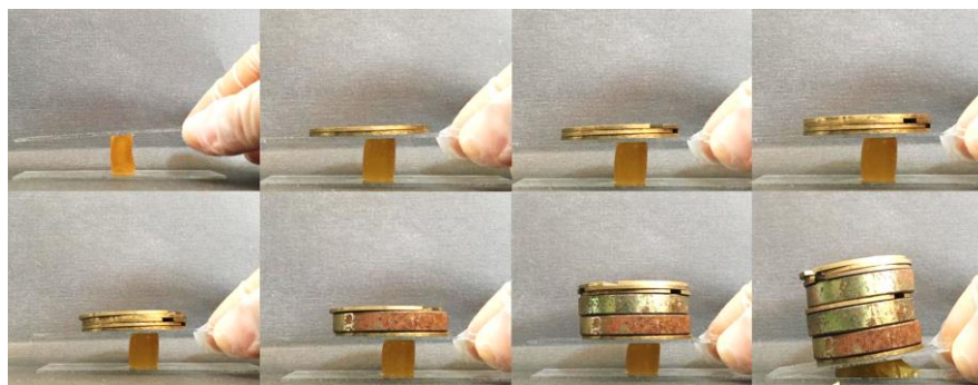
Figure 1. The compressive tests of the prepared samples
