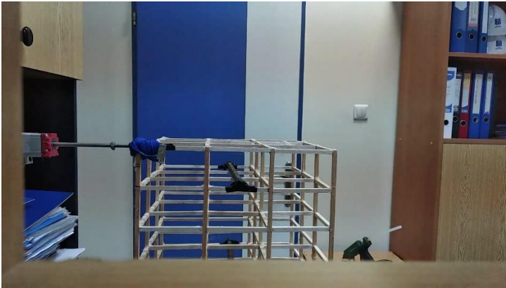
Figure 1. Displacement Meter Connection and Tracking Point
