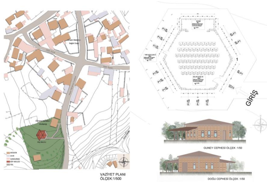
Figure 32. Library building site plan, plan and elevations
